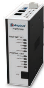
Anybus X-gateway in PROFINET IRT/PROFINET IRT combination
