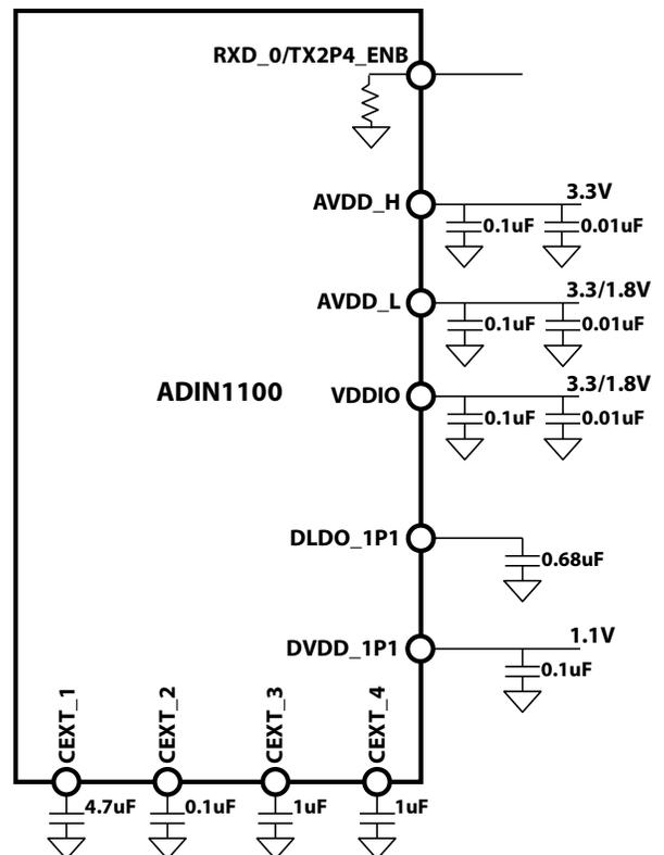
Figure 11. Supplies and capacitors for 2.4/1.0 V pk-pk transmit mode
