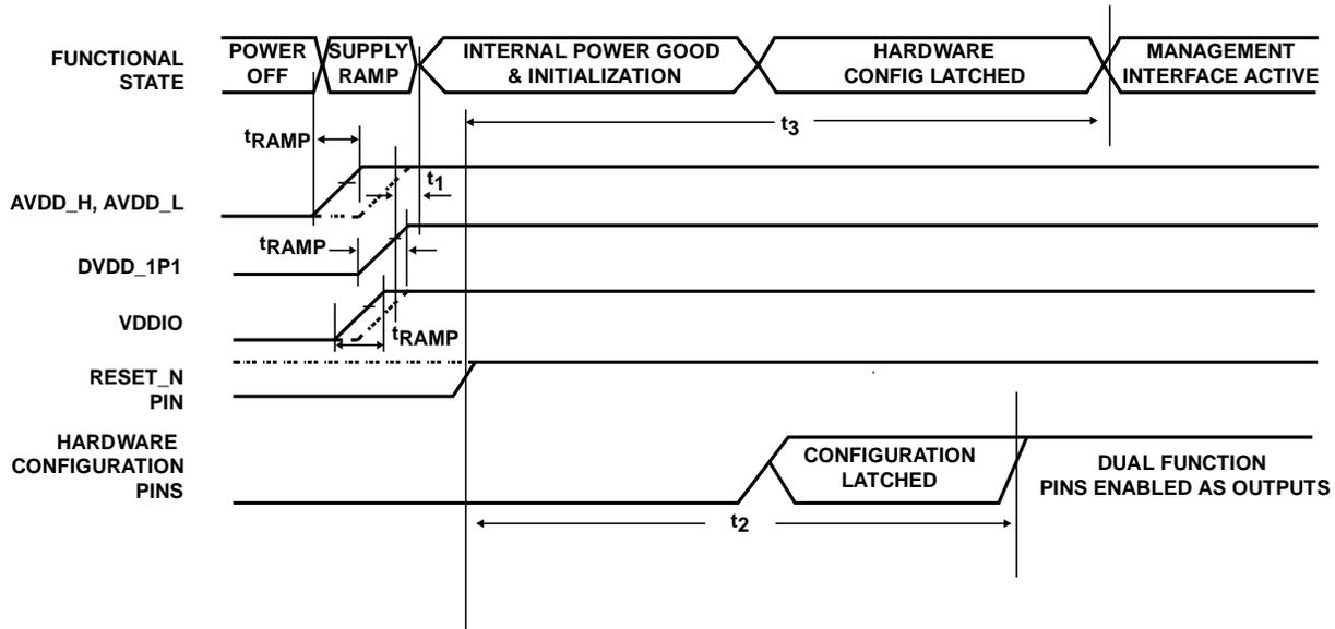
Figure 2. Power-Up Timing
