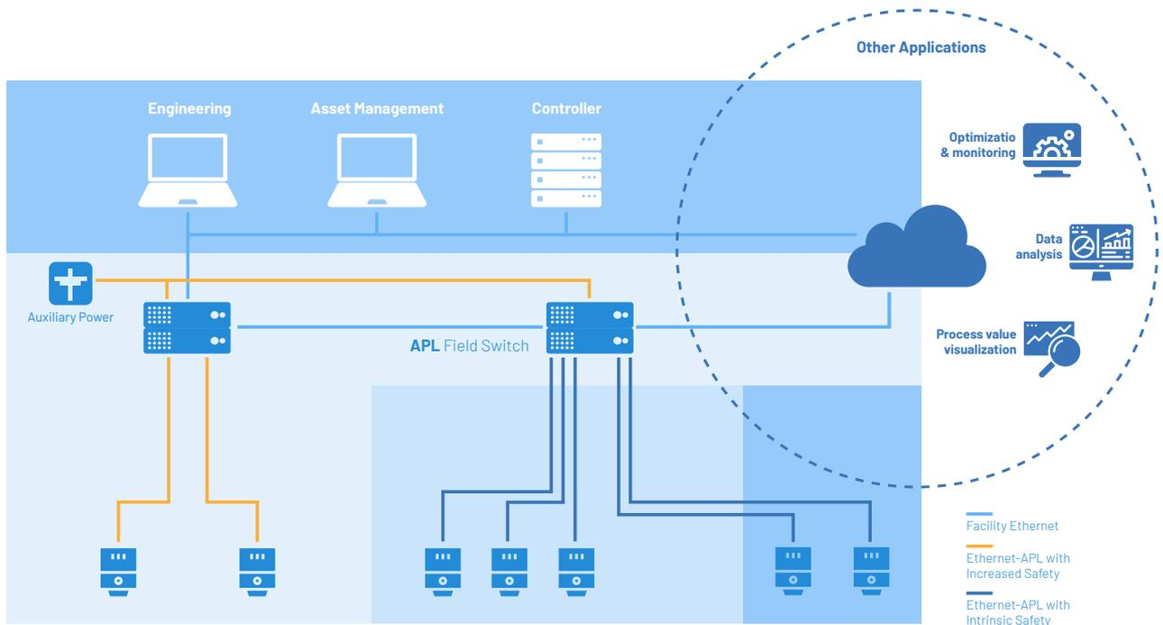
**Figure 6:** Networking the entire automation pyramid
